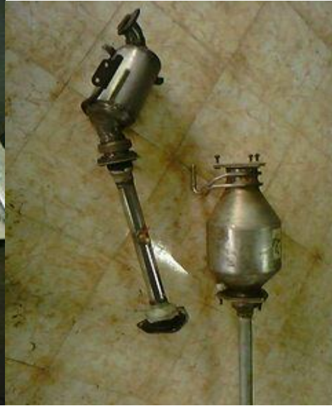
Figure 7: DPF and TWC Converters
